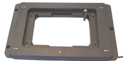
Custom Piezo-Z flexure stage, 200µm Travel, sub-nanometer resolution, millisecond response.
