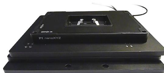
PInano™ XYZ piezo scanner mounted on a M-545.2P long travel, ultrasonic motor microscope stage. The XYZ piezo nanopositioning stages provide <1 nm resolution and are available with up to 200μm scanning range. The high stability and autolocking feature of M-545 provides significant advantages over other microscope stage designs when using fast piezo scanning stages. Request paper on long term stability!
